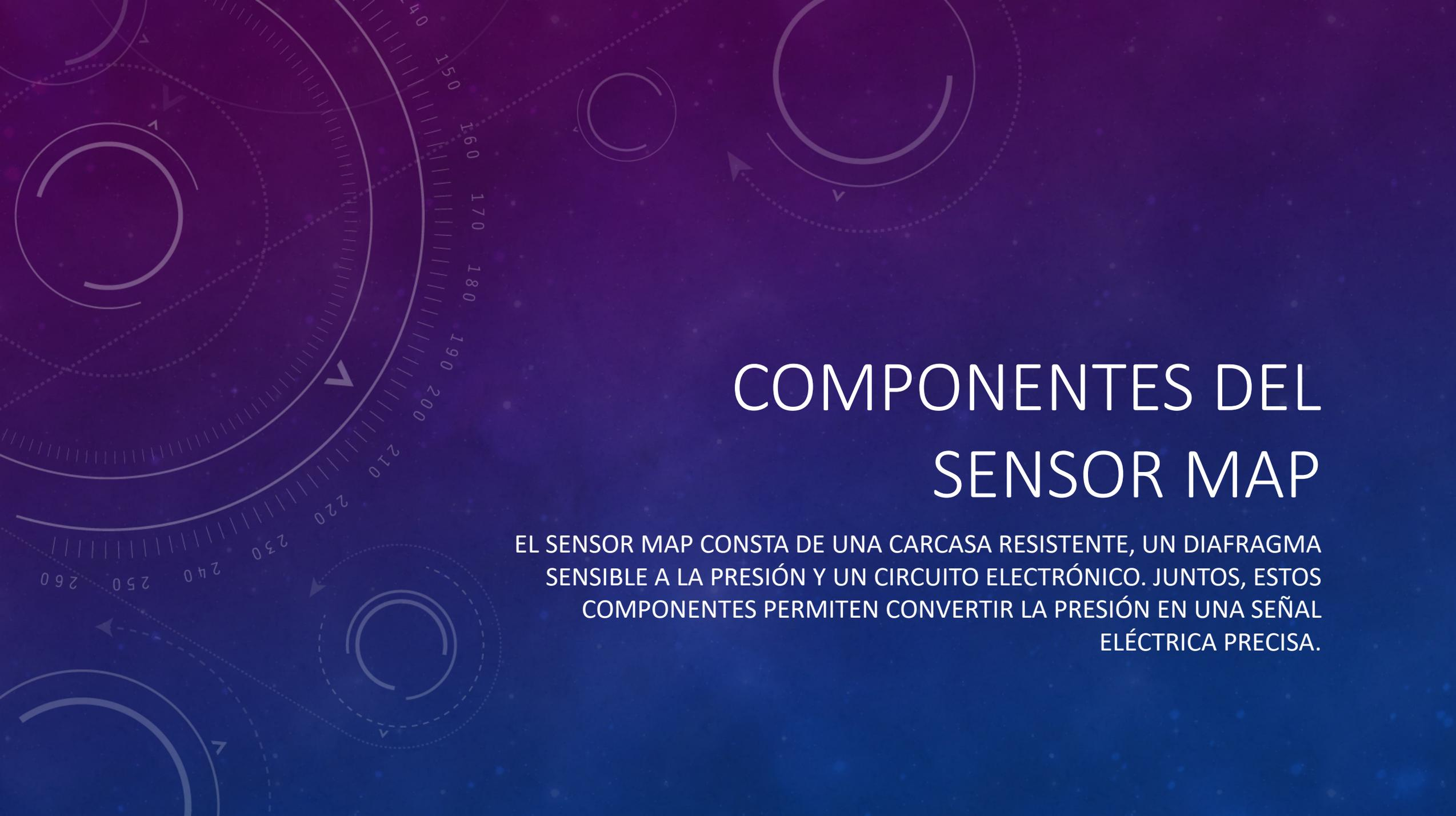
The background features a dark blue gradient with technical diagrams. On the left, a large circular scale is visible, with numerical markings from 140 to 260 in increments of 10. Several circular diagrams with arrows and dashed lines are scattered across the background, suggesting mechanical or electrical components.
